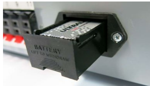
Figure 1 – Battery compartment (opened)
